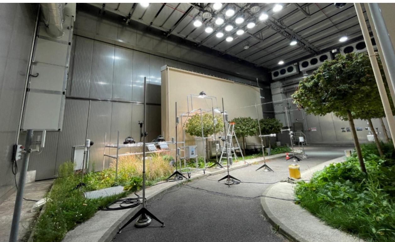
*Monitoring stormtrees and raingarden inside the SenseCity climatic chamber*
